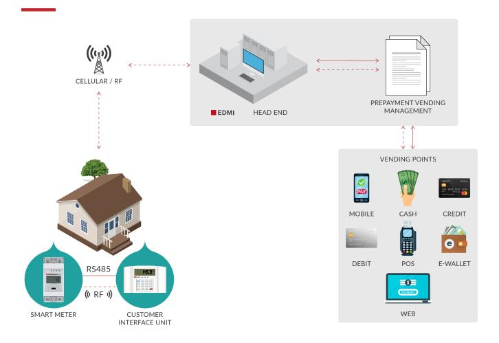
EDMI prepayment solution provides the end customer a seamless energy prepayment experience by integrating EDMI's meter, CIU and Head End system. With top notch meters coupled with different communication options (RF, Cellular, etc.) to meet different market requirements, real time communication in between the meters and head end software is assured. Various vending mediums such as POS, Web Mobile among others provide the end consumers the convenience for top-up and other transaction.
